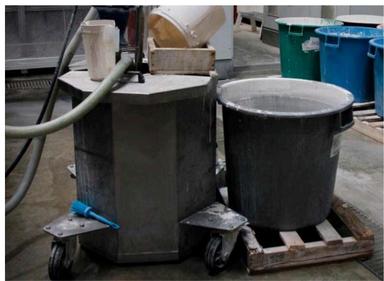
In the new production unit glazing machines have a suction system that allows the glaze to be reused. Vacuum system collect the glaze, dry it and transform it into powder, which is later reinserted into the production process.
